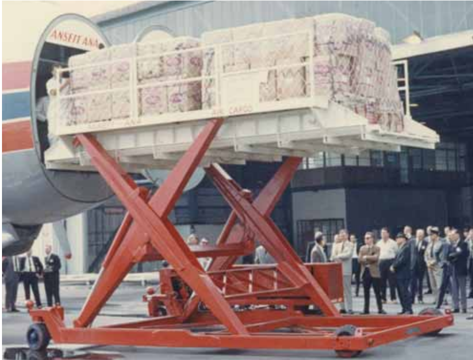
Ansett ANA Air Cargo Lift removing cargo from the nose of the aircraft.
